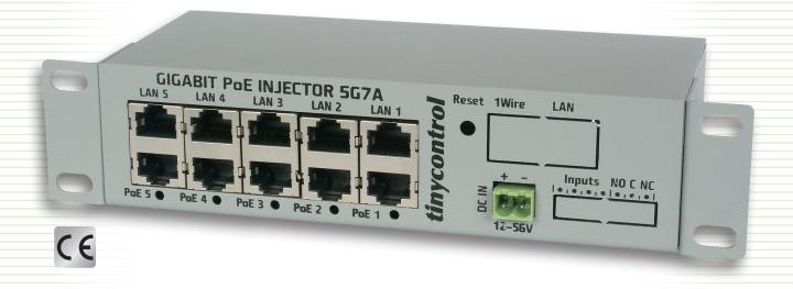
Gigabit PoE injector is manufactured in our company to the needs of operators, wireless internet. As the only passive PoE device can deliver up to 1.5A power supply cable Ethernet standard 1 Gb/s. This effect was achieved using special, high current transformers on signal lines ethernet manufactured in Poland for our order. Power signal is introduced only four lines in accordance with the passive PoE 100 Mb/s, so that the device is completely compatible with the slower version of the LAN.
